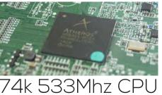
Powered by Qualcomm Atheros AR9344 Premium Wireless System on Chip (WiSoC) based on a the MIPS32 74K architecture
