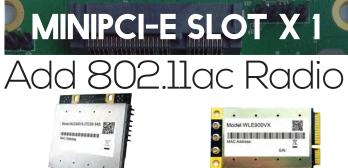
WPJ344 support a whole range of Compex 802.11ac miniPCI-e Radio Modules to enable Dual Band 11ac support for speeds up to 1300Mbps.
